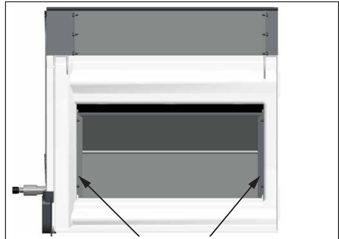
FIGURE 12: CM60C Horizontal Right Coil Condensate Final Assembly Upflow or Downflow Applications (CF/CM Models)
