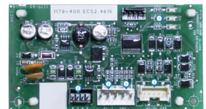
Indoor EEV Control
