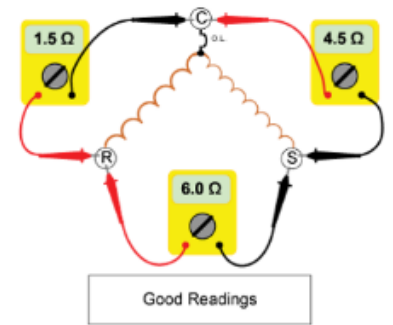
Example of Good Readings Between Terminals on Single Phase Compressor
