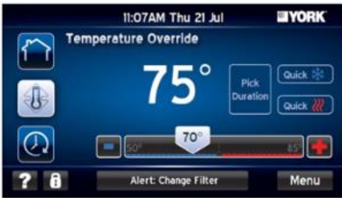
Temperature Override Screen - Advanced Programmable Mode
