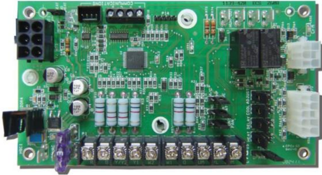
AVC/ MVC Control Board
