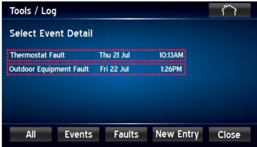
Tools / Log screen. When Enabled, Additional Event Detail May Be Viewed By Pressing The Fault.
