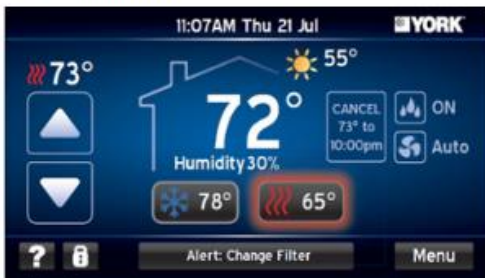
Home Screen Indicating Temperature Override & Heating Mode Active
