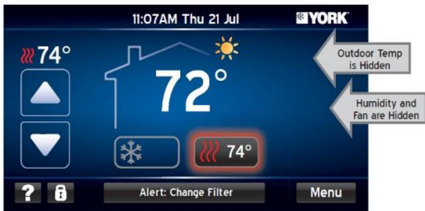
Home Screen With Selected UI Components Displayed - Outdoor Temp, Humidity & Fan Icons Are Hidden.
