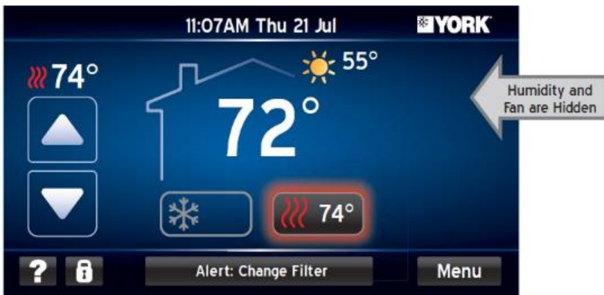
Home Screen With Selected UI Components Displayed - Humidity & Fan Icons Are Hidden.
