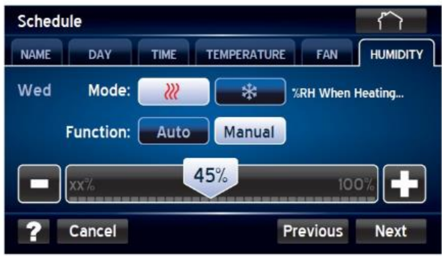
Humidity Settings May Be Established For Each Programmable Time Period (Manual Mode Illustrated Here)
