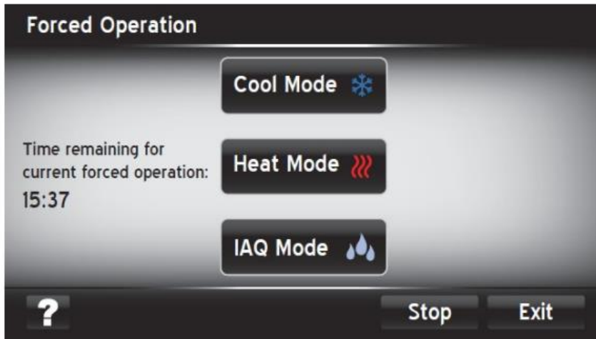
Time Remaining In Current Forced Operation Mode Is Displayed.
